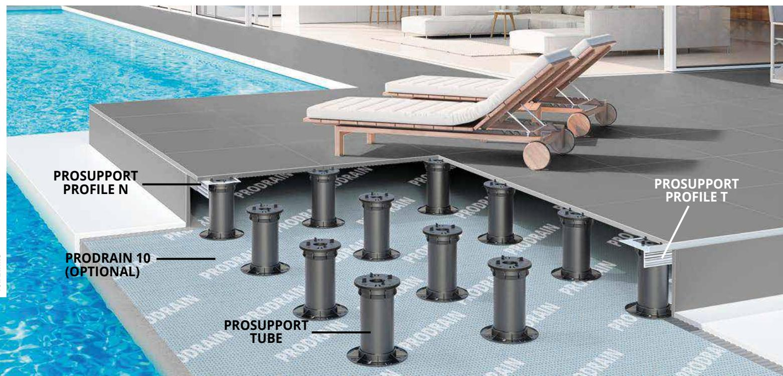
**PROSUPPOR PROFILE T & N** is a profile for the protection and finishing of the external edge of raised floors in ceramic, wood and composite materials. The vertical section of the profiles features a specially designed fins that create a dovetail cladding system. This dovetail cladding system allows for the adhesive used to fix the covering to also mechanically bond to the profiles. The profile is also available with a decorative edge of 2 cm height (PROSUPPOR PROFILE T).
