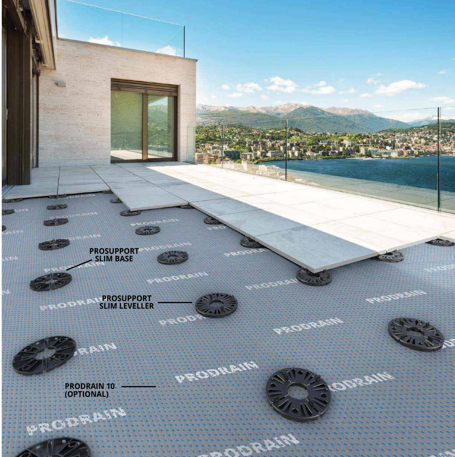
**SUPPORT** and **LEVELLER** are suitable for the realization of outdoor floating floors. The support, in polyethylene, has a height of 15 mm. The rubber leveller, with a thickness of 3 mm, can be applied on the supports up to a maximum of 2. **SUPPORT** and **LEVELLER** are suitable for outdoor areas, terraces, pool edges and pedestrian crossings.
